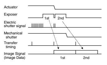
Figure 3 Timing chart of using full frame CCD.
