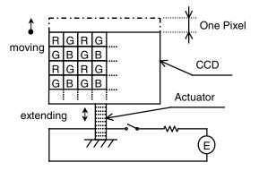
Figure 2 One-dot-movement mechanism.
