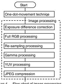
Figure 4 Flow chart of image processing.
